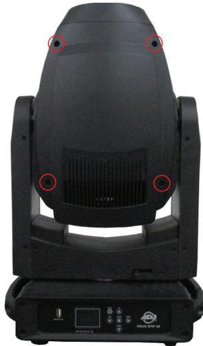
2. Locate the gobo wheels and color wheels. They are positioned near the second large silver thumb screw on each side of the head. Turn the color wheel to that the open slot is facing towards you, and then turn the gobo wheel until the gobo you wish to replace is aligned with the open slot of the color wheel.
